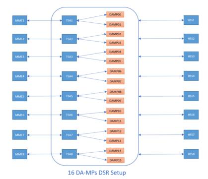
Figure 3-1 DA-MP Relay Testing Topology
